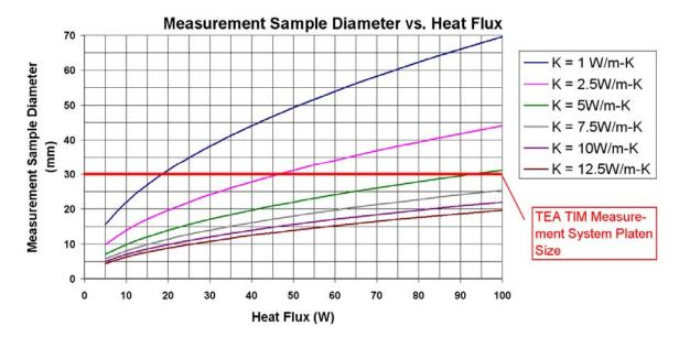
Using this graph, one can either find a value of D for a given Q or, conversely, a value of Q for a given D for values of  $K_{\theta}$  in the 1 to 12.5W/m-K range. Equation 3 should be used for greater  $K_{\theta}$  values. Equation 2 should be used for square measurement samples.
